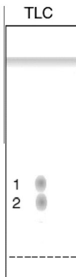
Figure 1 Separation of 1-TFP and 2-PCP by TLC method (methanol as mobile phase).
