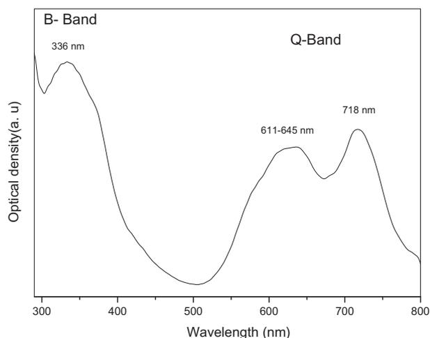
**Figure 2** Absorption spectrum of Cu-Pc/PS thin films.
