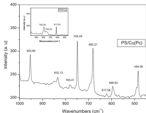
**Figure 5** Raman spectra of Cu-Pc/PS thin films.
