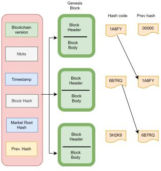
Figure 4. Structure of the Blockchain Header
