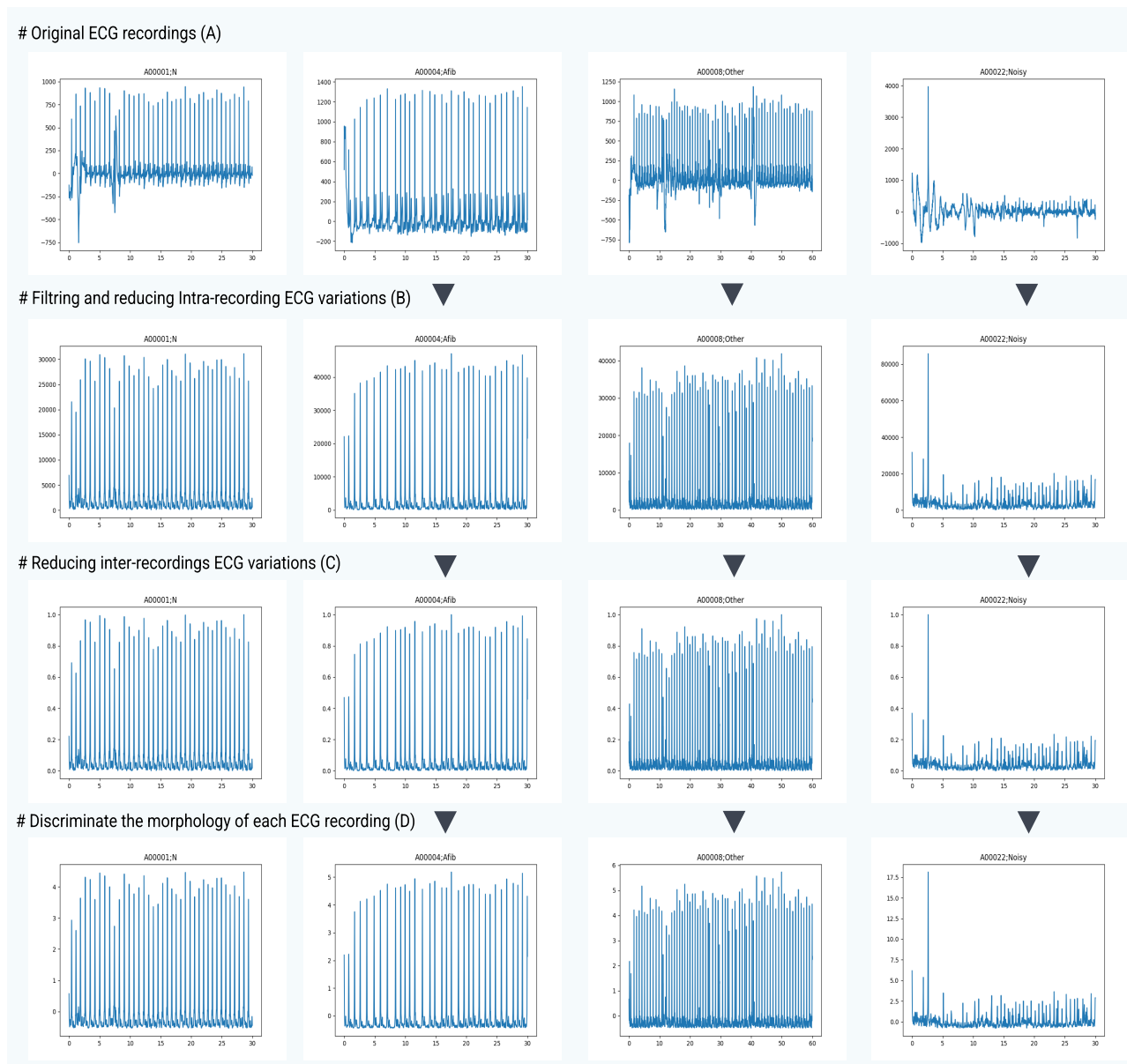
Figure 2. Illustration of the preprocessing steps applied to ECG signals from the CinC2017 dataset, demonstrating the transformation of recordings from Normal (N), Atrial Fibrillation (AF), Other rhythms, and Noisy categories. Panels (A) show the original ECG recordings. Panels (B) illustrate the effect of filtering and reducing intra-recording variations, showcasing the signal smoothing and noise reduction. Panels (C) depict the process of reducing inter-recording variations, standardizing the signal amplitude across different recordings. Finally, panels (D) demonstrate the discrimination of the morphology of each ECG recording, highlighting the morphological consistency achieved before segmentation. These visualizations collectively underscore the comprehensive preprocessing strategy employed to enhance signal quality and consistency for subsequent analysis.
