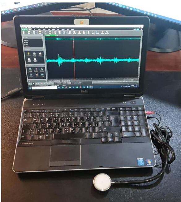
Figure 2: Stethoscope Built for Data Recording
