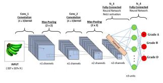
Figure 10. Phase of Classification that is Proposed for Banana Grading in the Food Processing Industry
