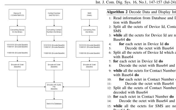
Figure 1. Encoding Information With Base64 Algorithm
