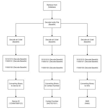
Figure 2. Decoding Information with Base64 Algorithm
