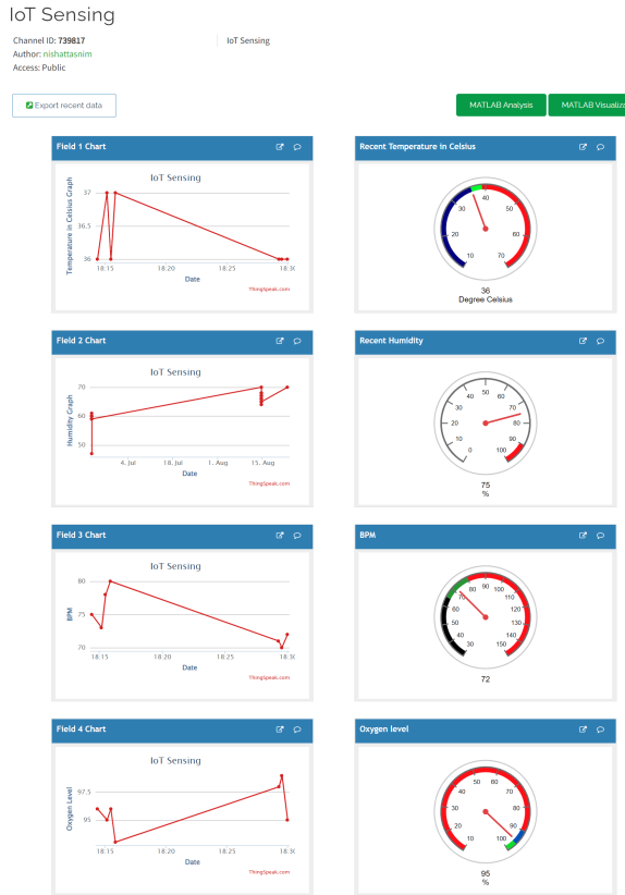
Figure 13. Collected data are uploaded to the cloud server automatically from Node-MCU via Wi-Fi which can be monitored, downloaded, and analyzed.
