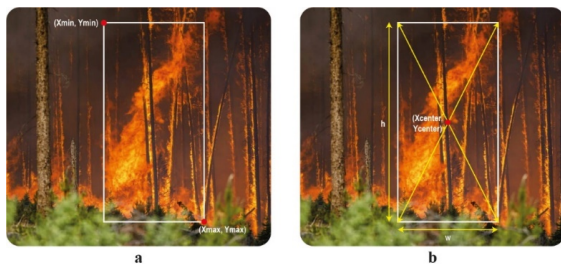
Figure 3. Regular vs YOLO annotation styles (a) Regular style (b) YOLO style
