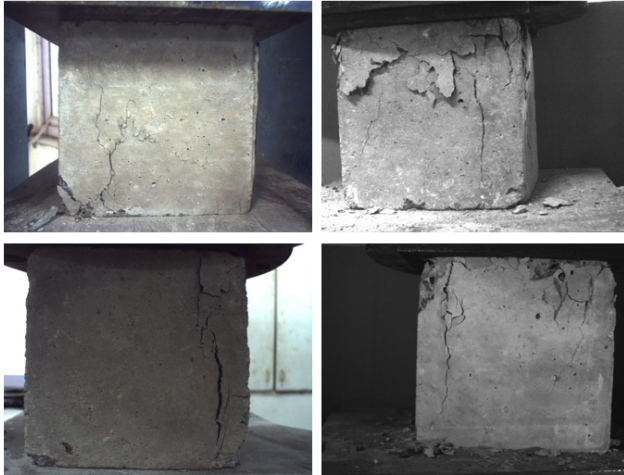
Figure 2. Concrete cube surface images without illumination and experimental setup
