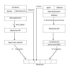
Figure 6. A simple BC-based security level evaluation mechanism for IoT.
