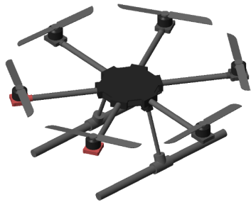
Figure 12. BIRD Simulink© SimScape© Multibody model
