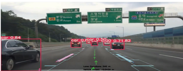
(c) Vehicle Detection on Highways with Improved YOLOv4+HNEM
