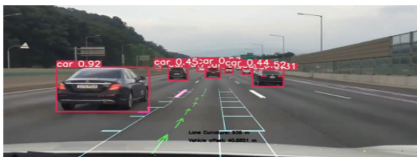
(a) Vehicle Detection in Normal Condition using YOLOv4 and HNEM
