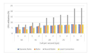
Figure 11. CPU Utilization measurement results on VOIP service
