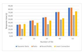
Figure 7. Response time measurement results on FTP Service
