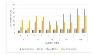
Figure 9. CPU Utilization measurement results on FTP Service
