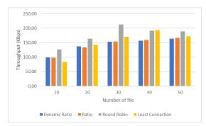
Figure 6. Throughput measurement results on FTP Service
