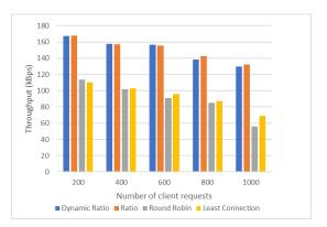
Figure 2. Throughput measurement results on web service
