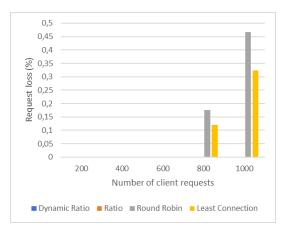
Figure 4. Measurement results of request loss on web service
