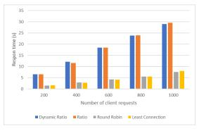
Figure 3. Measurement results of time response on web service
