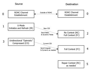
Figure 17. ROHCv2 Context Setup in Unidirectional mode [117]
