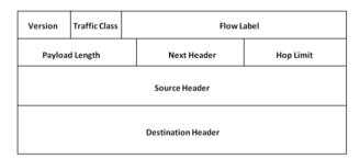
Figure 4. IPv6 packet header format [37]
