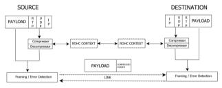
Figure 13. Application of ROHC in a protocol stack [112]
