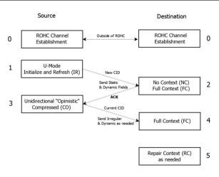
Figure 18. ROHCv2 Context setup in Bidirectional mode [117]
