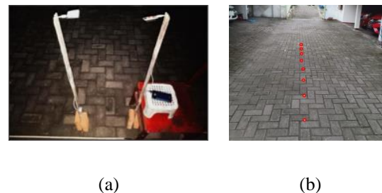
Figure 11. The measurement setup for RSSI values vs distance
