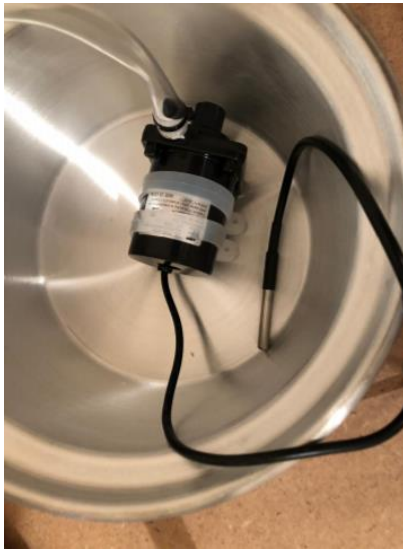
Figure 9. Pump inside the container
