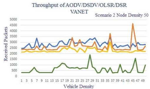
Figure 5. Throughput of different Routing protocol for node density of 50
