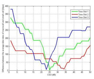
Figure 3. Selection of optimum CSO values in three different time slots.
