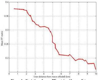
Figure 1. Variation of mean PF metric with user distance from macro eNSodeB.
