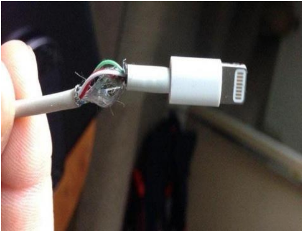
Figure 1. Frayed Charging Cable.
