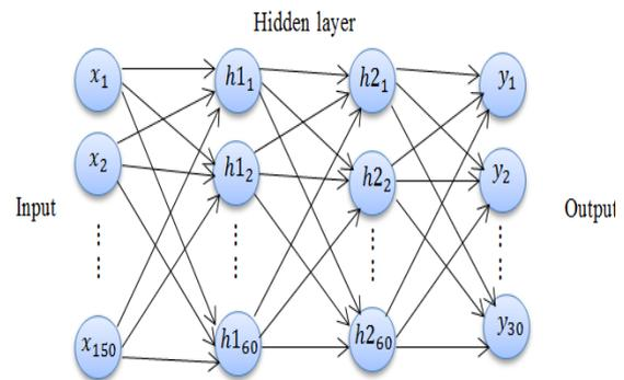
Figure 5. Architecture for BP neural network
