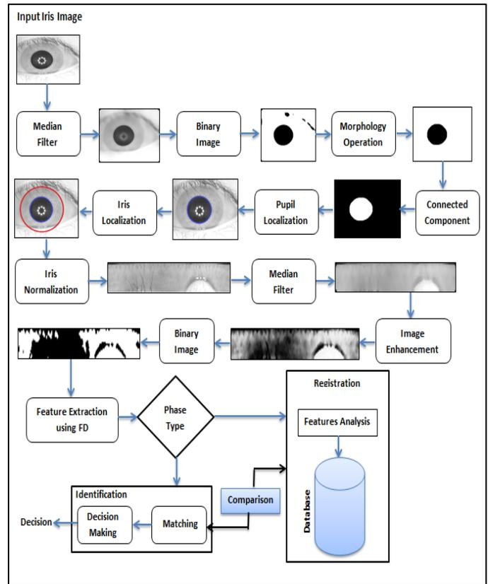
Figure 6. The proposed system procedure.
