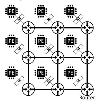
Figure 1. Standard NoC components.
