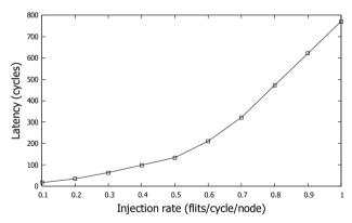
Figure 4. Latency measurements for simulation of  $2x^2$  cluster of 4  $2x^2$  NoC-based systems.
