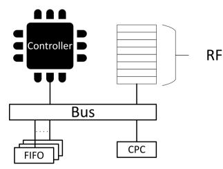
Figure 6. ICFIFO internal structure in  $NoC^2$ .
