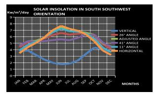
Figure 14. Solar Insolation in Bahrain for various tilt angles in southwest orientation
