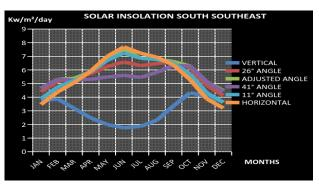
Figure 15. Solar Insolation in Bahrain for various tilt angles in southeast orientation
