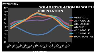
Figure 13. Solar Insolation in Bahrain for various tilt angles in south orientation
