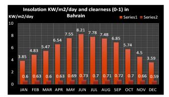
Figure 12. Solar insolation and purity of the horizon in Bahrain
