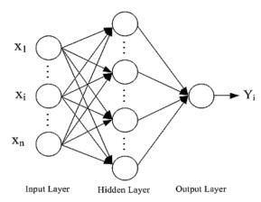
Figure 2. Multi-layer perceptron Neural Network.
