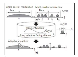
Fig. 1. Comparison of SCM and MCM: (a) frequency spectra of transmitted signals; and (b) frequency spectra of received signals, after [1].
