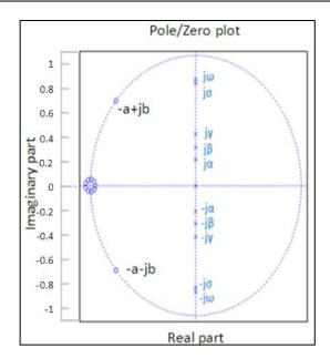
Fig.8. Pole-zero plots for 11th order intermediate IIR half-band filter.
