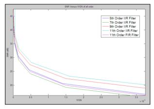
Fig.13. SNR Versus AWGN for 5th, 7th, 9th, 11th FIR and 11th IIR filter order for BLWDFBs.
