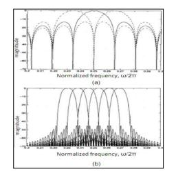
Fig.4. Frequency responses of six spectrally contiguous subchannel pulse sequences: (a) DMT transmission; (b) DWMT transmission, after [4].
