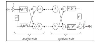
Fig.7. Lattice structure realization of the IIR wavelet filter bank, after [17].
