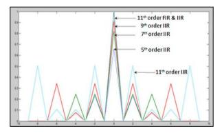
Fig.14. Autocorrelation functions for 5<sup>th</sup>, 7<sup>th</sup>, 9<sup>th</sup>, 11<sup>th</sup> order IIR -BLWDF and 11<sup>th</sup> order FIR filters.
