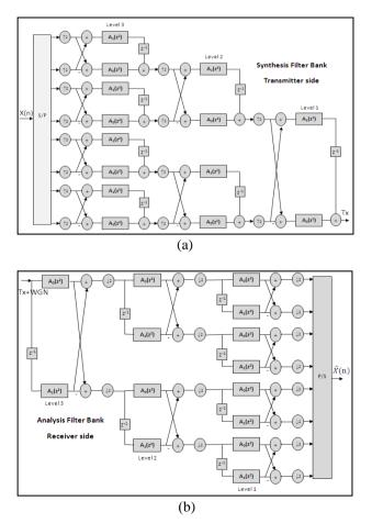
Fig.12. Block diagram of (a) the proposed DWMT transmitter, (b) the proposed DWMT receiver.
