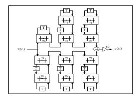
Fig. 5. An 11th-order lattice wave digital filter, after [15].
