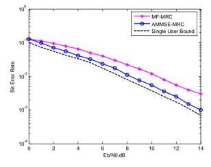
Fig. 6. BER vs SNR performance of proposed adaptive MMSE-MRC detector in multipath channel, M=3 paths, G=32
