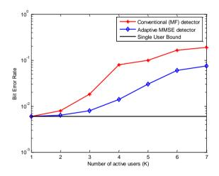
Fig. 3. A performance comparison of the adaptive MMSE detector with conventional and single user case for different system load in AWGN. G = 32, Eb/No = 5dB
