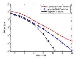
Fig. 2. A performance comparison of the adaptive MMSE with conventional and single user case in AWGN channel. G = 32, K = 3 users
