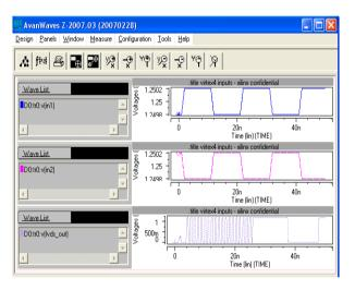
Fig. 4. Comparator action of differential pin at reduced swing and 50  $$\rm MHz$$
