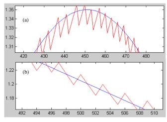
Fig. 9. Capacitor voltage tracking the input signal (a) at positive peak (b) at zero crossing
