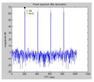
Fig. 11. FFT for two tone input signal
