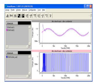
Fig. 8. Comparator output of SD-ADC
