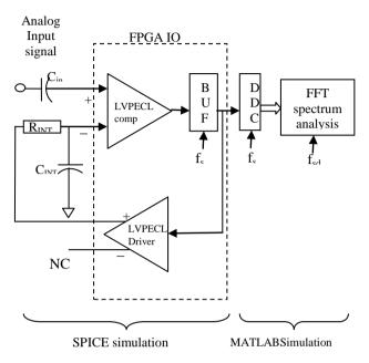
Fig. 5. Block diagram of SD-ADC used for simulation
