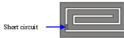
Figure 4. Disconnect the spiral resonator.
