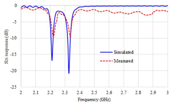
Figure 17. Simulated and measured  $S_{21}$  of the manufactured multi-resonator tag with code "110".
