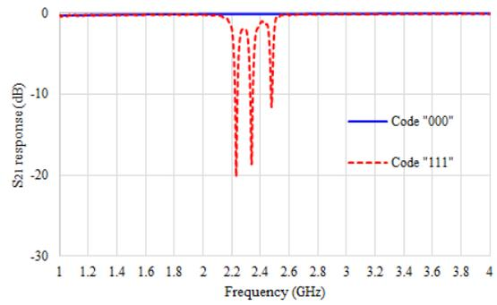
Figure 10. Simulated  $S_{21}$  of the designed multi-resonator tag with different codes "000" and "111".
