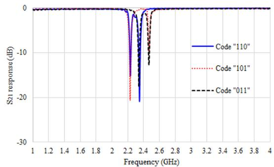
Figure 12. Simulated  $S_{21}$  of the designed multi-resonator tag with different codes "110", "101" and "011".
