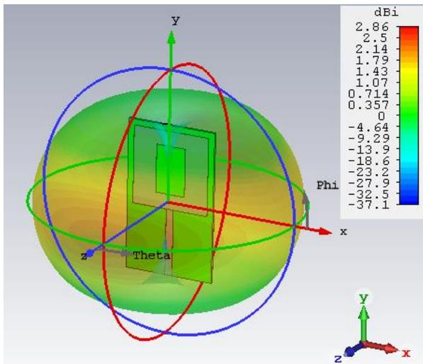
Figure 9. Radiation pattern of the monopole antenna at 2.5 GHz.
