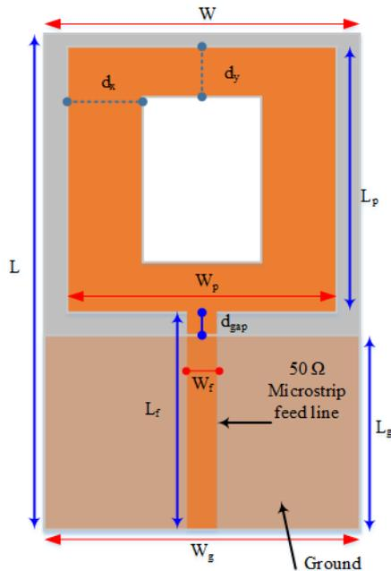
Figure 2. UWB monopole antenna [10].
