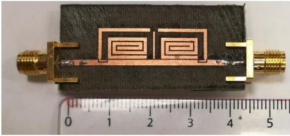
Figure 13. Photograph of the RFID chipless tag.
