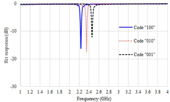
Figure 11. Simulated  $S_{21}$  of the designed multi-resonator tag with different codes "100", "010" and "001".
