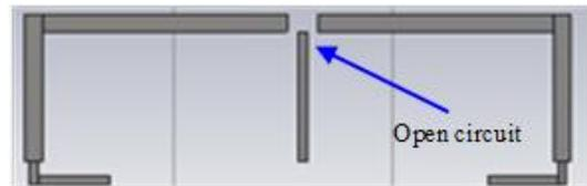
Figure 5. Disconnect the coupled line by an open circuit.
