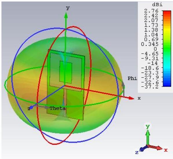
Figure 8. Radiation pattern of the monopole antenna at 2.36 GHz.
