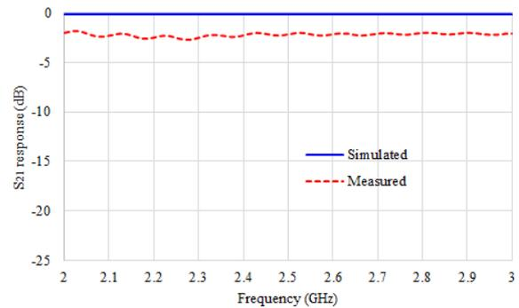
Figure 16. Simulated and measured  $S_{21}$  of the manufactured multi-resonator tag with code "000".
