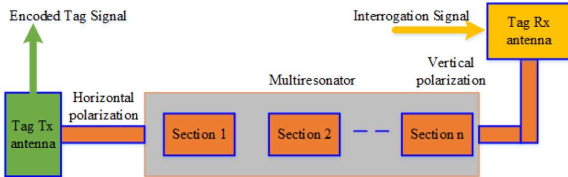
Figure 1. Geometry of chipless RFID tag [9].
