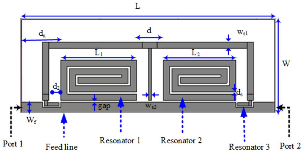
Figure 3. Geometry of the multi-resonator structure.
