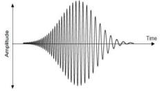
Figure 1(b). The Gaussian pulse (chirped)
