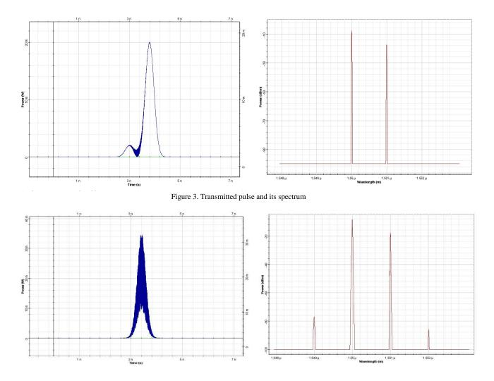
Figure 4. The transmitted pulse and its spectrum for 60 Km transmission distance
