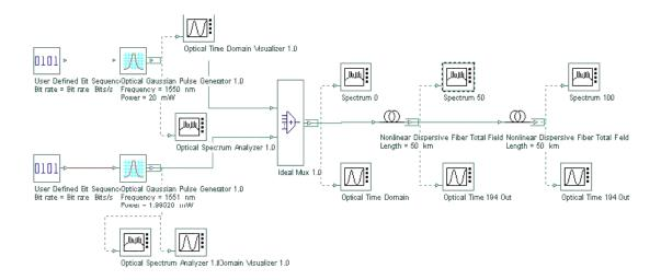
Figure 2. Optical fiber communication project design
