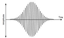
Figure 1(a). The Gaussian pulse (un-chirped)
