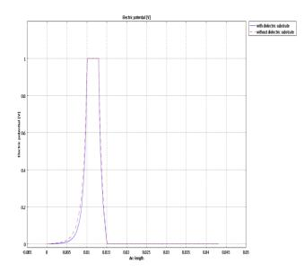
Figure 10. Comparison Analysis of Potential distribution of the model with and without dielectric substrate
