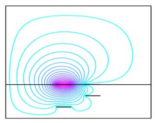
Figure 4. Contour plot of the potential distribution of unshileded fourconductor transmission lines.
