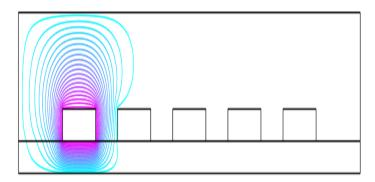
Figure 9. Contour plot of the potential distribution of the unshielded fiveconductor transmission lines.
