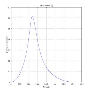
Figure 5. Potential distribution of unshielded four- conductor transmission lines using port 1 as input along a line from (x,y) = (0,0) to (x,y) = (10, 10) mm.
