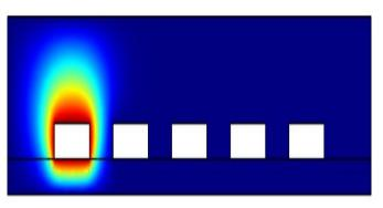
Figure 7. 2D surface potential distribution of the unshielded five-conductor transmission lines.
