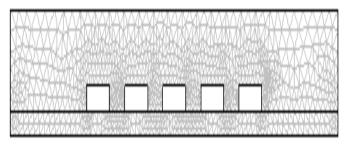
Figure 8. Mesh plot of the unshielded five-conductor transmission lines.
