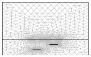
Figure 3. Mesh plot of unshielded four-conductor transmission lines.
