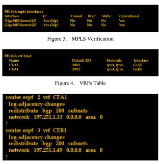
Figure 5. CE-PE OSPF routing
