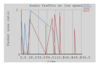
Figure 7. Packet-Loss Rate in Audio Traffic at low speeds
