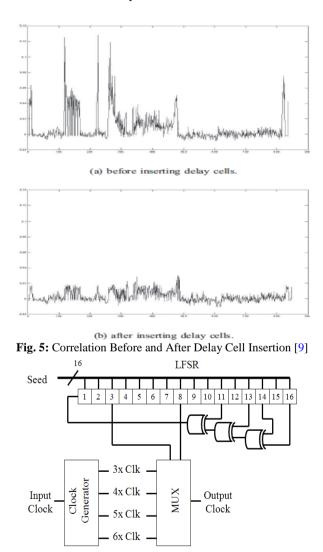
Fig. 6: Random Clock Countermeasure Module
