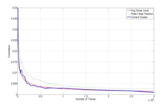
Fig. 8: DPA Results Based on Number of Traces for Randoml Clocked AES
