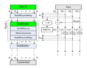
Fig. 10: System Level Bit Balancing Design
