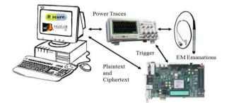
Fig. 2: Experimental Setup
