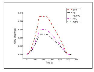
Figure 3. Concentration of carbon dioxide in MCR at  $20^\circ\!\text{C}$
