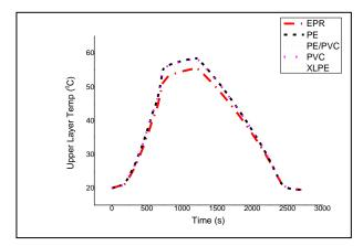
Figure 1. Upper layer temperature in MCR at 20°C
