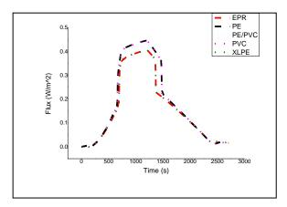
Figure 7. Fire sizes of targets (cables) in MCR at 20°C
