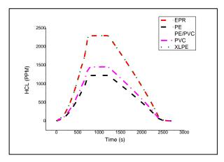
Figure 4. Concentration of hydrogen chloride in MCR at 20°C
