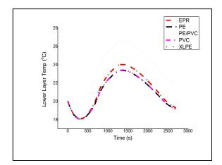
Figure 2. Lower layer temperature in MCR at 20°C
