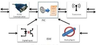
Fig. 5: ISM block diagram.
