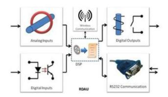
Fig. 2: RDAU block diagram.
