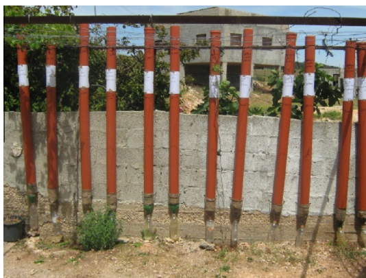
Figure 2 Experimental setup for the soil columns.
