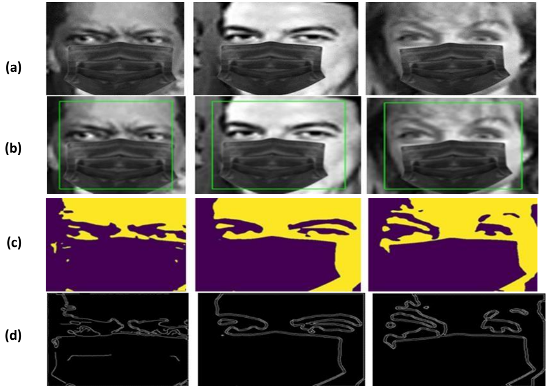
Figure 3: Sample images of a human face with an emotion (a) input images (b) Face detected image (c) Patch generated image (d) Edge detected image
