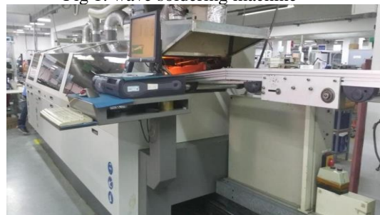
Fig 2. the gateway of wave soldering machine
