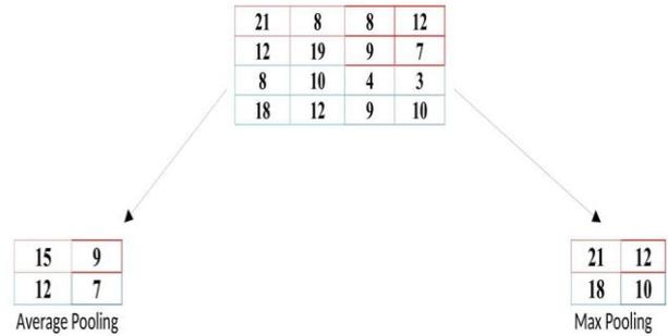
Figure 4. Average Pooling and Max Pooling
