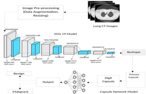
Figure 8. Architecture of the VggCapNet
