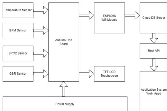
Figure 2. Diagram of Hardware System Components.
