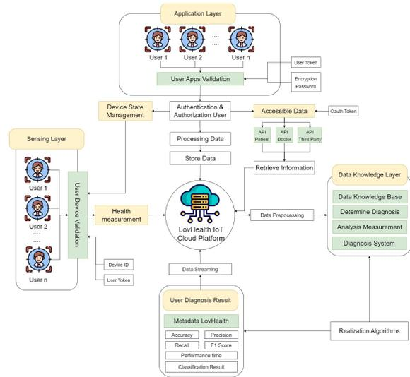
Figure 9. Flow diagram Cloud Centric IoT Diagnosis Systems.
