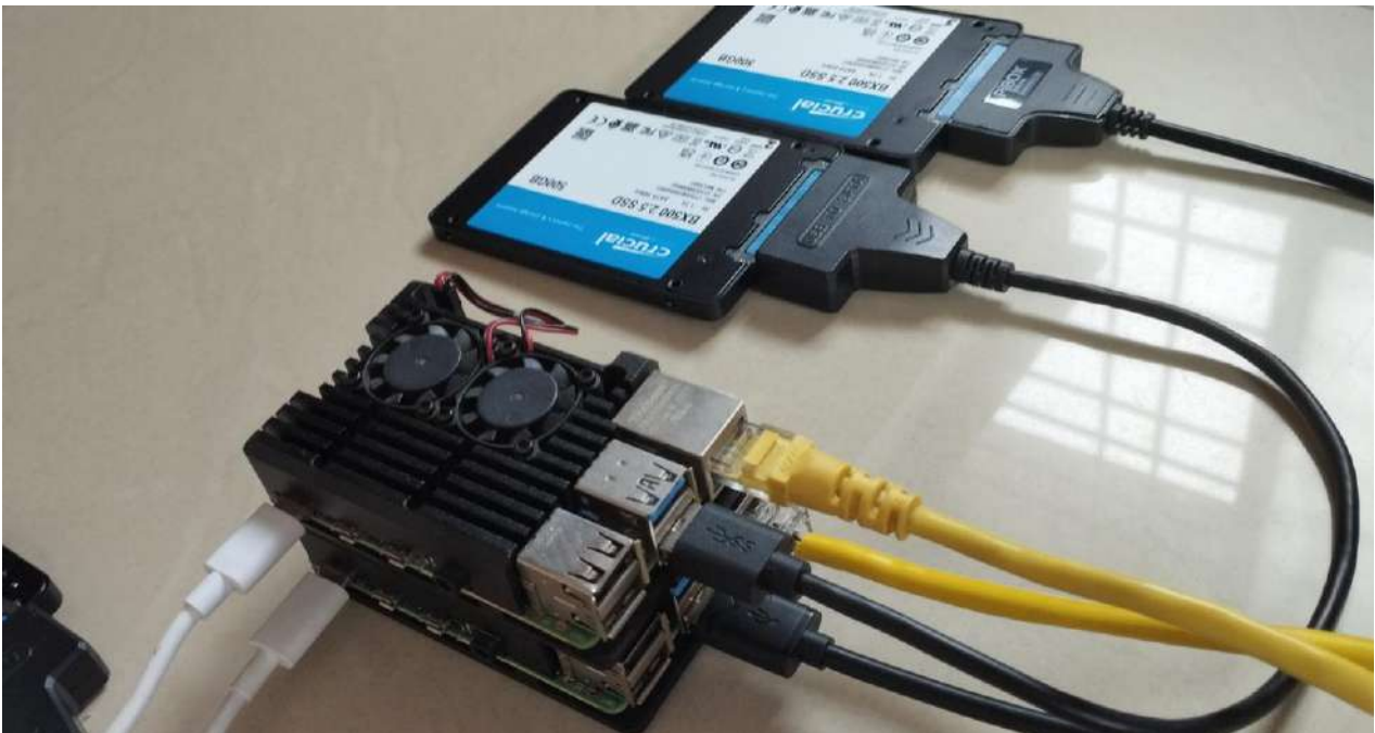
Fig 1c. Edge Cluster power usage is typically around 45W at peak processing demand
