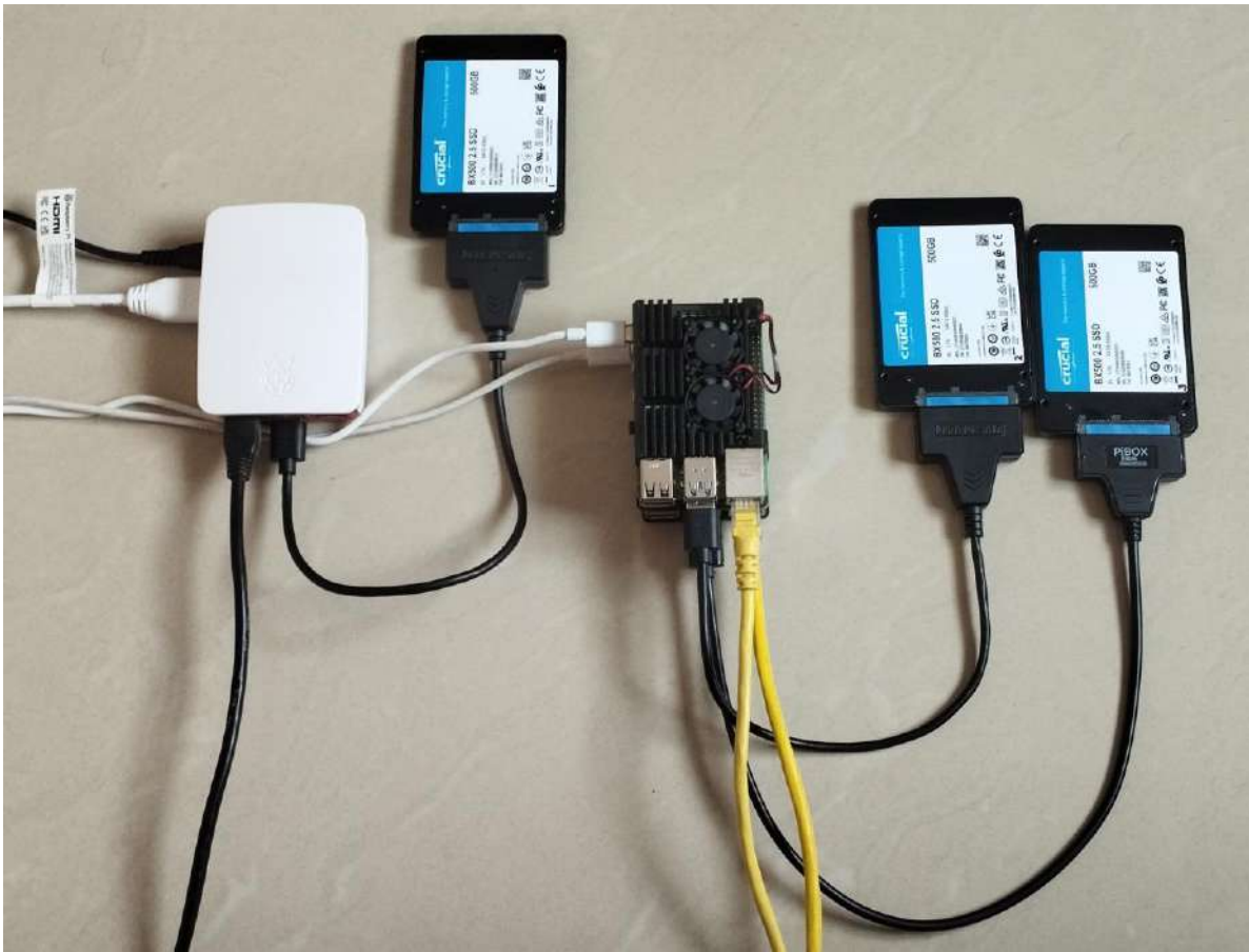
SBC cluster connections with two RPi 4 – 8GB and one RPi 3B+ Storage Controller
