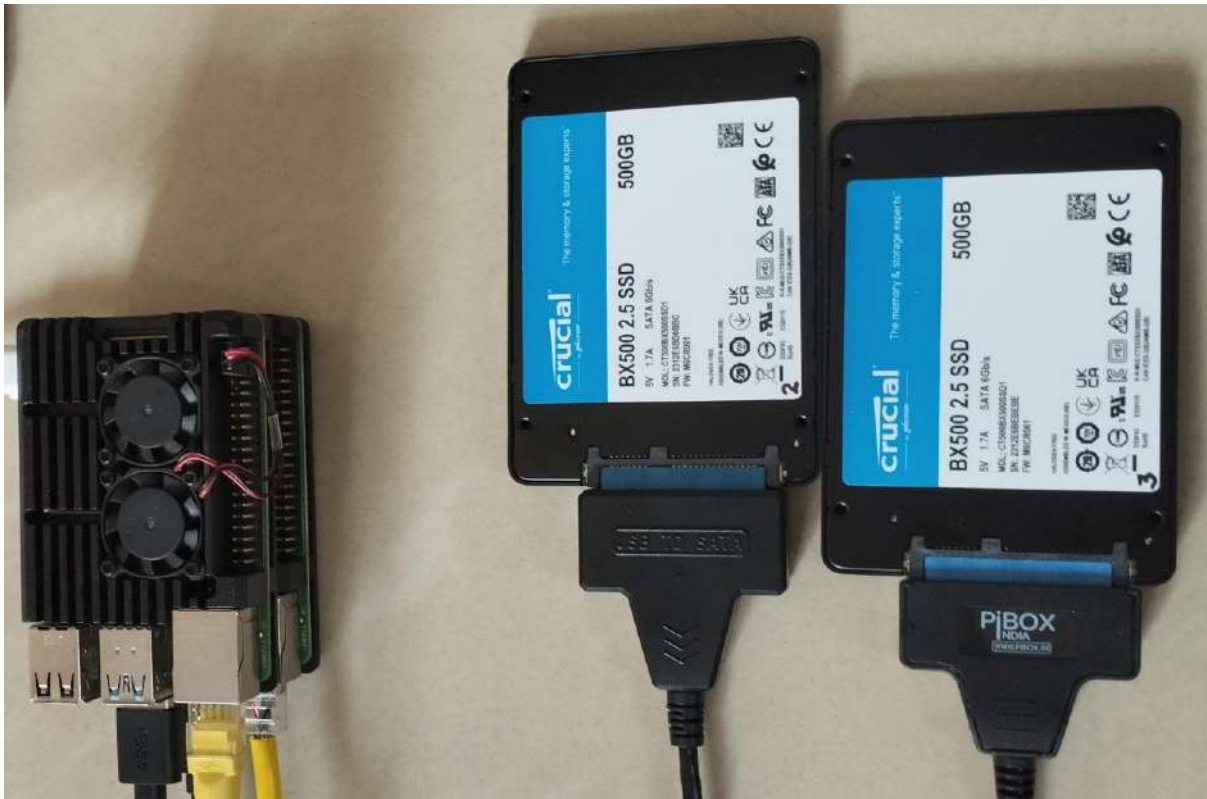
Fig 1b. USB SSDs ensure quick bootup and optimal edge performance with 300Mb/s throughput
