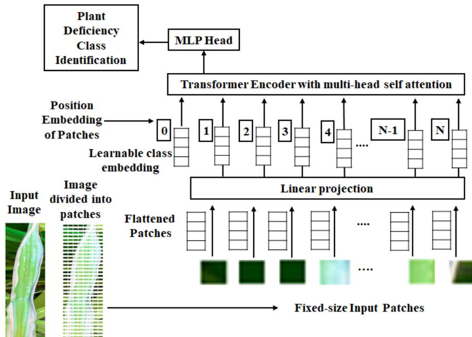
Figure 3. Vision transformer model [44]
