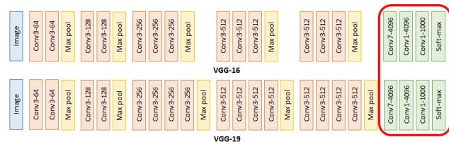
Figure 6. VGG16 and VGG19 Architectures
