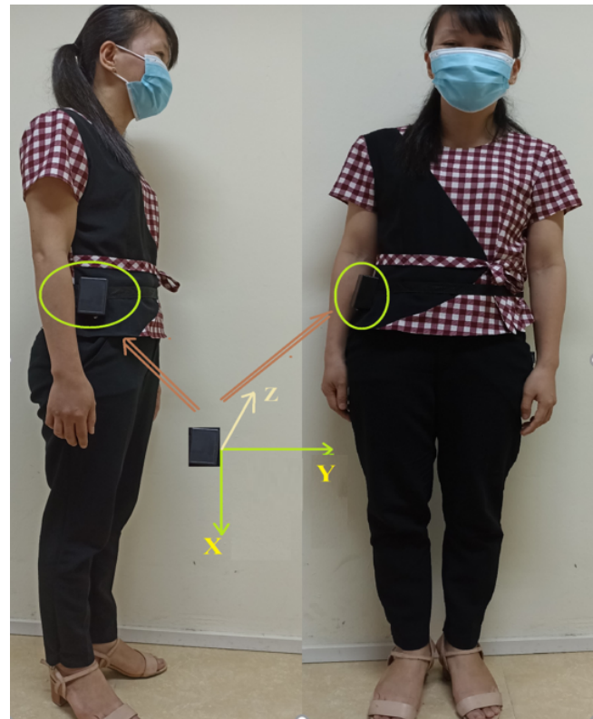
Figure 4. Location of monitoring equipment
