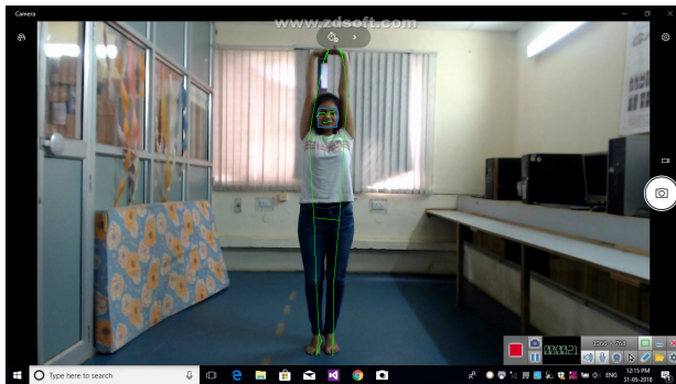
Figure 4. Tadasana pose detected by Blaze Pose
