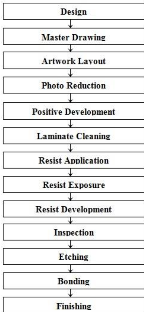
Figure 13. Flowchart for steps involved in Patch antenna fabrication
