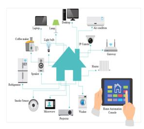
Figure 5. Typical IoT Smart Home Architecture
