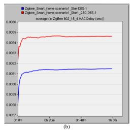
Figure 15. TStar topology comparison in global mode for 1ZC and 2ZCs (a) Throughput (b) Delay
