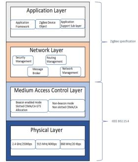
Figure 2. ZigBee Layers
