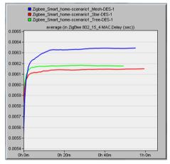
Figure 10. End-to-end delay for 1ZC ZigBee network in global mode
