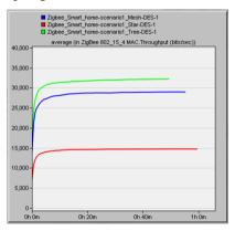
Figure 8. Average throughput for 1ZC ZigBee network in global mode
