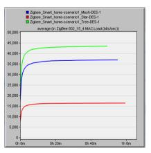
Figure 9. Average load for 1ZC ZigBee network in global mode
