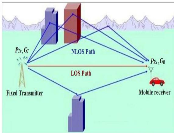
Figure 2. A typical mmWave communication Scenario.
