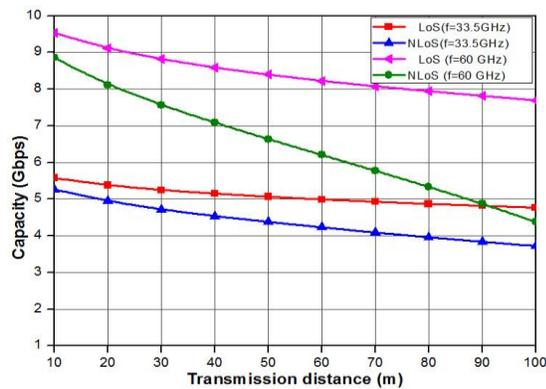
Figure 7. Capacity at 33.5 and 60 GHz for LOS and NLOS cases.
