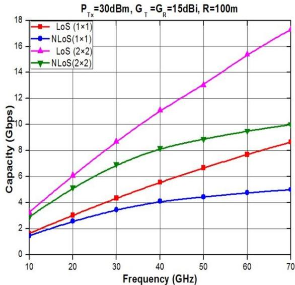
Figure 4. Data carrying Capacity as function of frequency
