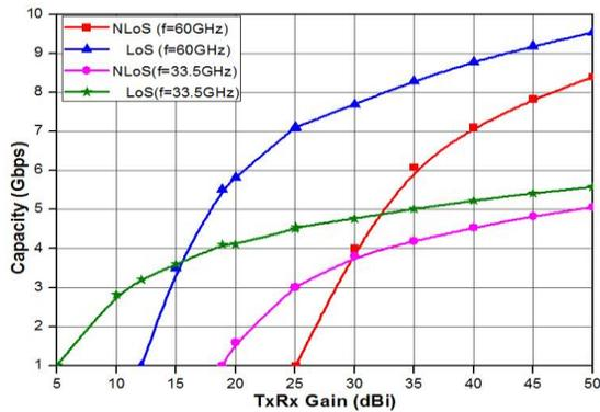
Figure 6. Capacity as function of combined transceiver gain
