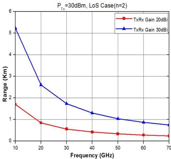
Figure 3(a). Range as function of frequency (LOS Case)
