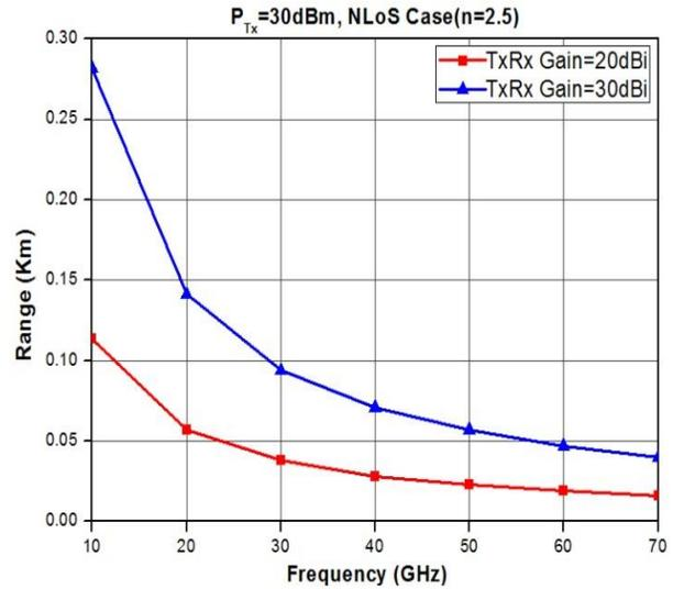
Figure 3(b). Range as function of frequency (NLOS Case)
