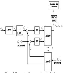
Figure 3.Generator side converter control scheme
