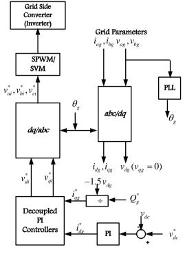
Figure 4. Grid side converter control scheme
