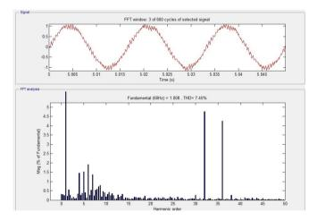
Figure 11. THD of Grid Current in PMSG based WECS
