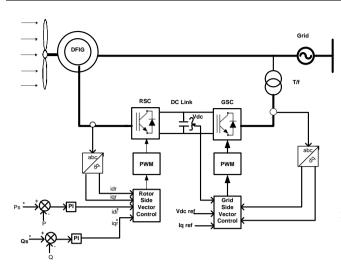
Figure 1. Block diagram of DFIG based Wind Energy Conversion System
