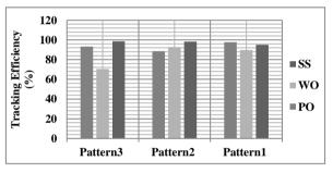
Figure 11. Tracking efficiency of various MPPT techniques
