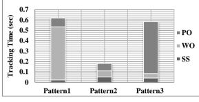
Figure 10. Convergence (Tracking) time of various MPPT techniques
