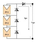
Figure 3. 3S PV array configuration.
