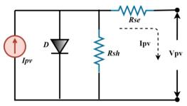
Figure 1. Equivalent circuit of the PV cell.
